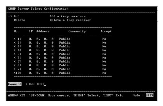
8. Arrow down to Trap and hit enter. This screen allows the user to send Traps about the iSwitch to ten IP Addresses (not required). Also, you may determine the severity levels and what type of access, read only or
